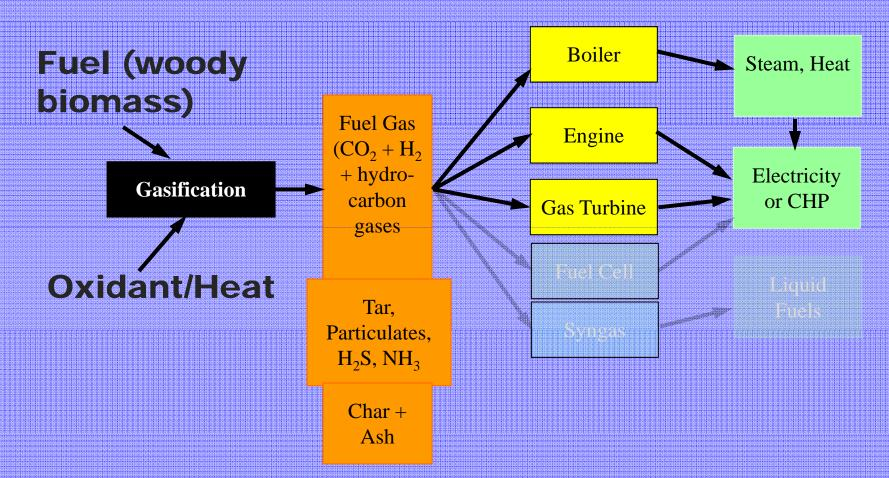
Gasification is the "Partial Oxidation" (controlled amount of air or oxygen) to produce a combustible, gaseous mixture (producer gas) of many compounds that can be used directly as a low BTU fuel gas or cleaned and used to produce higher value products (syngas). Moderate Scale Combined Heat and Power (CHP) Gasification Unit.
